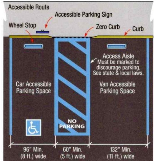
Note: Van parking spaces can be 96" (8 ft.) wide Min. if the access aisle is 96" (8 ft.) wide Min.
